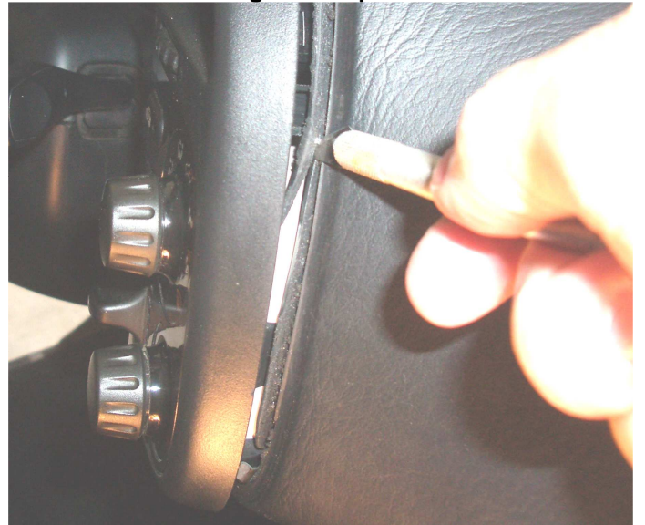
Photo 2 – Trimming excess plastic flush with dash
