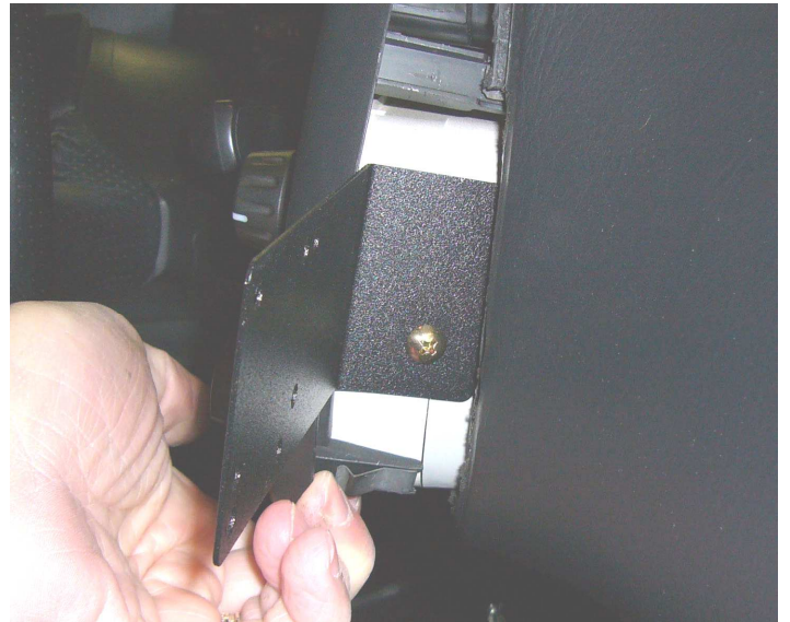
Photo 4. Bracket mounted using heater control screw
